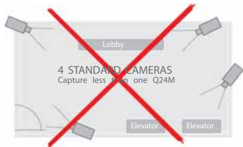
Hemispheric room cover- age for a wall mounting - one Q24M replaces four standard cameras
