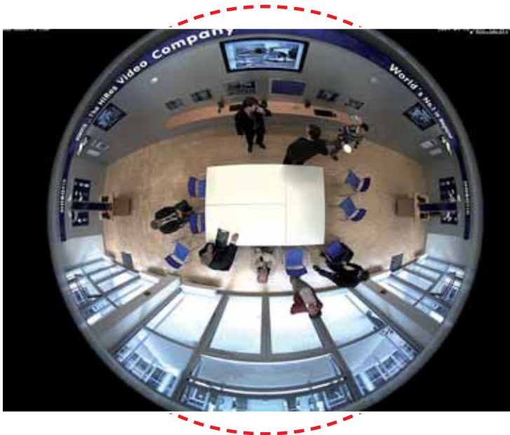
Original full image from the Q24M (ceiling installation in a rectangular room)
